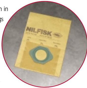
The electrostatic paper bag offers finer filtration capabilities, retaining 97.8% of particles down to 1.5 microns. Its electrostatically charged inner lining is comprised of meltblown polypropylene to attract ultra-fine particles, enabling the bag to capture materials such as toner.
